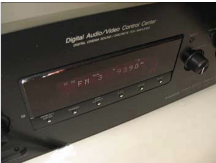
The plastic front panel of a modern AM/FM stereo receiver can be a source of RF interference.
