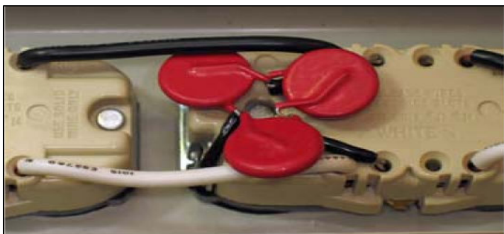
This power strip contains three MOVs, or metal oxide varistors. The MOVs absorb electrical surges that exceed the normal 120 volts AC
